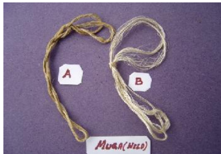
Muga yarn of wild variety of A. assama (a) Som fed (b) Mejankari fed cocoon
