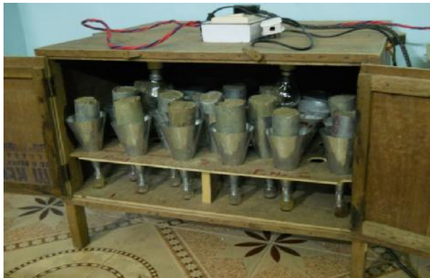
Plate No.4 b: Arrangement of funnels along with soil sample
