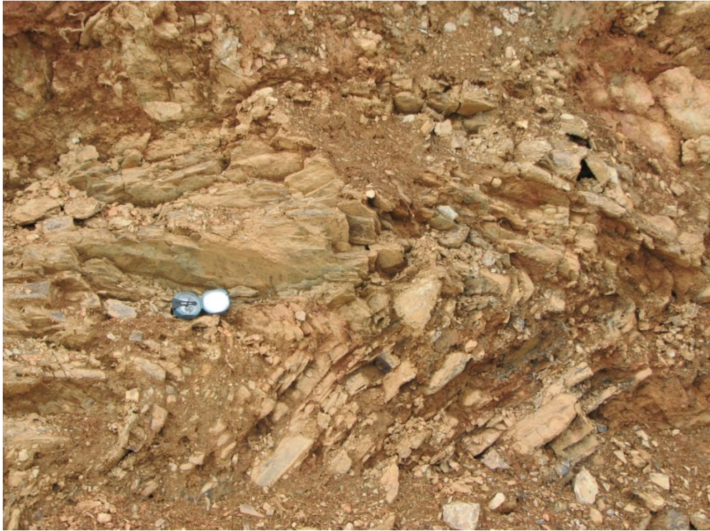
Plate 8.1. Folding in shale
