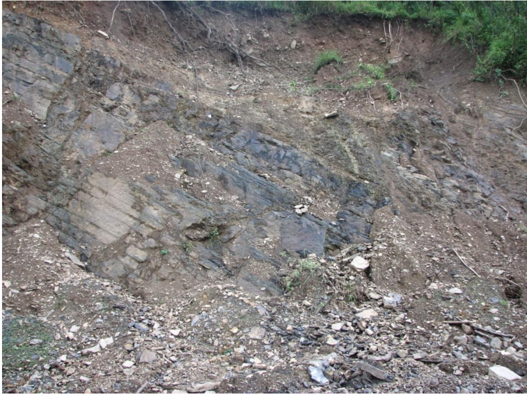
Plate 7.9a. Partially weathered shale capped by weak soil
