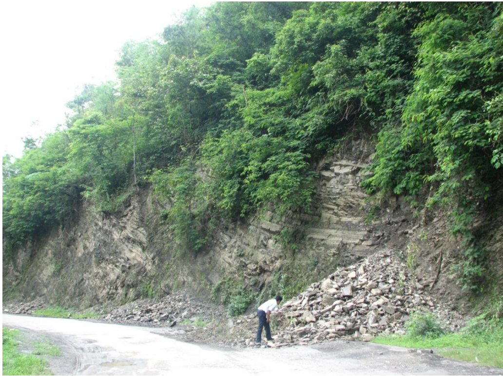
Plate 7.4a. Jointed and fractured rocks
