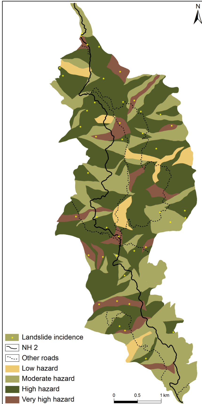
Fig. 6.1a. Landslide hazard zonation map
