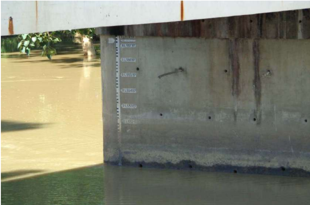
Plate 2: Water level measuring station of Kakodonga River at National Highway 37 crossing point
