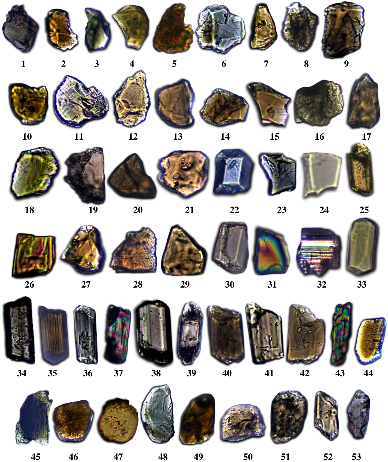
Plate 19: Observed heavy minerals; (1-21) anhedral; (22-45) euhedral to subhedral and (46-53) subrounded to rounded tourmaline with and without inclusions
